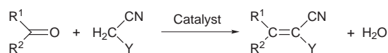
Scheme 2 Knoevenagel condensation of different carbonyl compounds with malononitrile or ethyl cyano acetate
